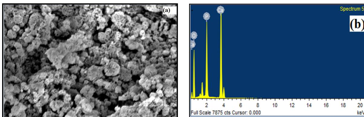
**Figure 2.** (a) FESEM image of HAp powder (b) EDX of Hap
